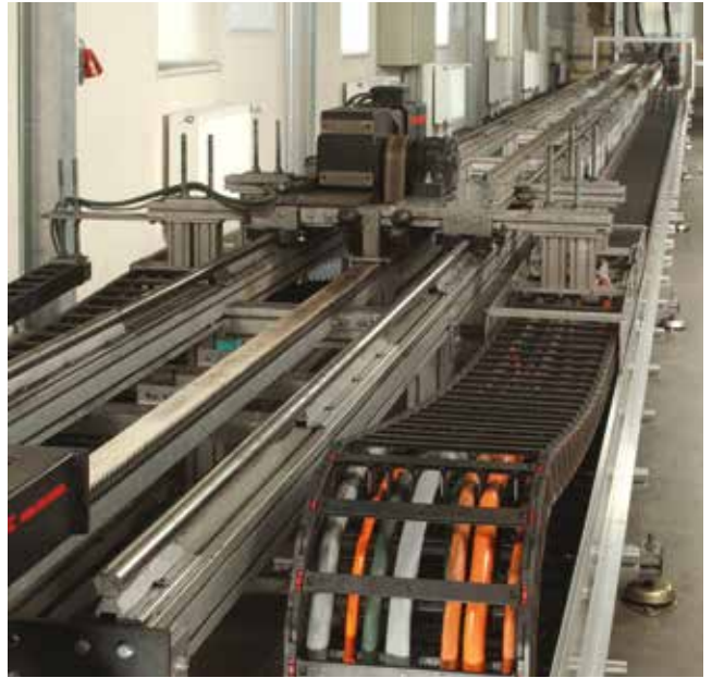
18 m drag chain test facility
