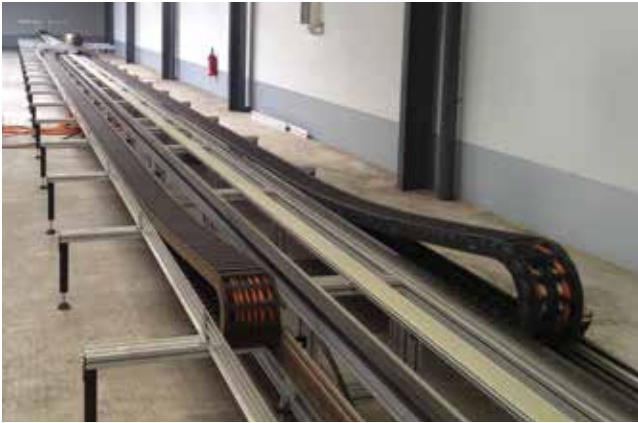
40 m drag chain test facility
