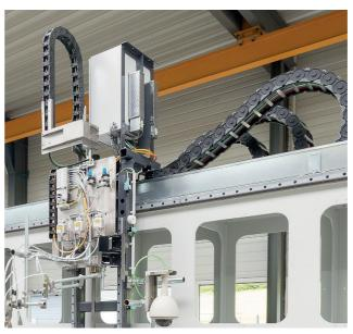
Drag chain systems are used for a wide range of applications and travel distances. EKD Systems has the right solution for every application: from self-supporting drag chains for short distances to gliding drag chains for longer distances. Our range also includes special slide shoes to reduce wear and channel systems to guide the chains. Even for very long movement distances and high additional loads, the MARATHON system is a reliable solution.
